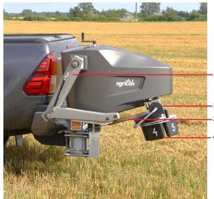
Fig. 2. Semi-automatic soil sampling equipment: 1 – automatically operated mechanical hand; 2 – needle cleaning mechanism; 3 – needle for taking soil samples from a depth of 20-30 cm; 4 – soil sample collection boxes
