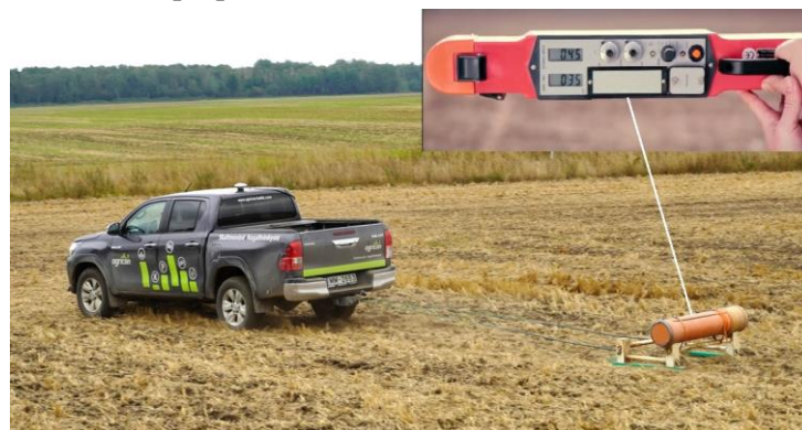
Fig. 1. Determination of soil electrical conductivity (ECa) with EM38-MK2 scanner
